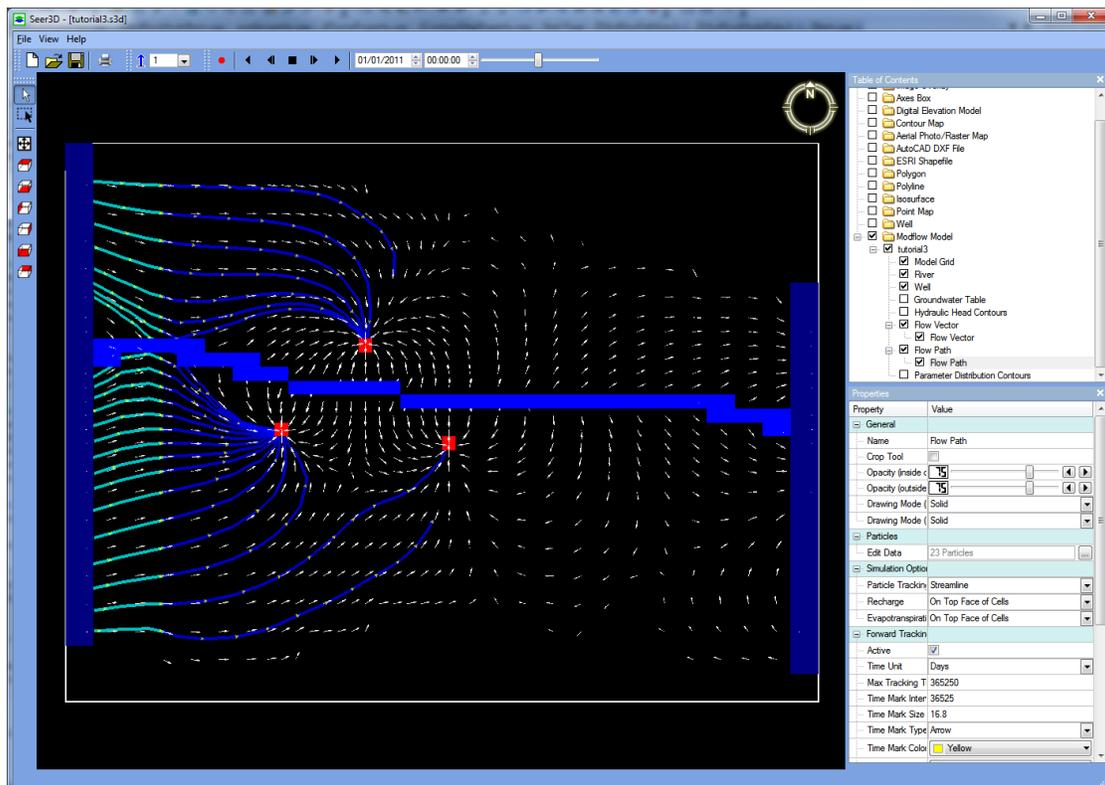
Figure 3.8. Flow paths of a model depicting the upstream capture zones of three pumping wells
