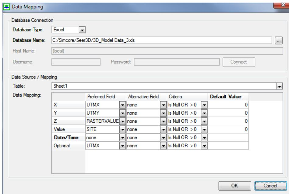
Figure 2.20. The Data Mapping dialog box for scattered data
