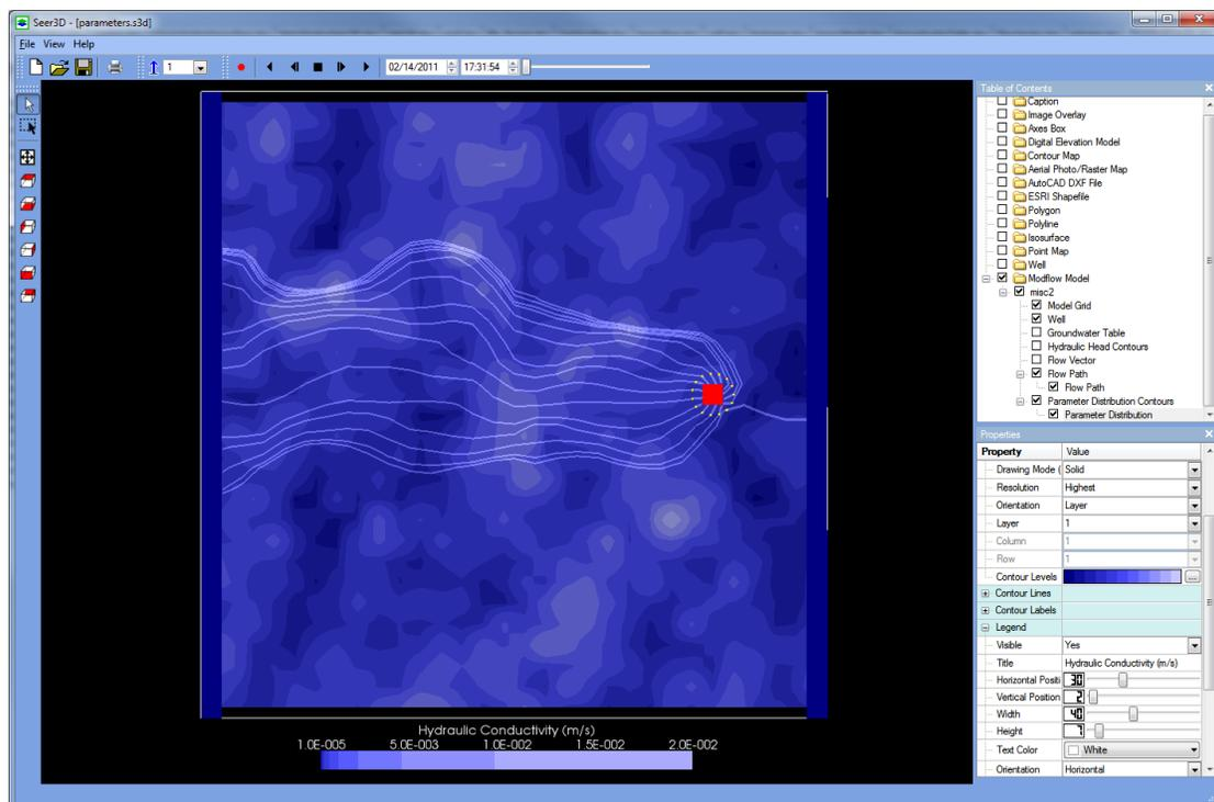
Figure 3.11. Streamlines and the distribution of hydraulic conductivity values
