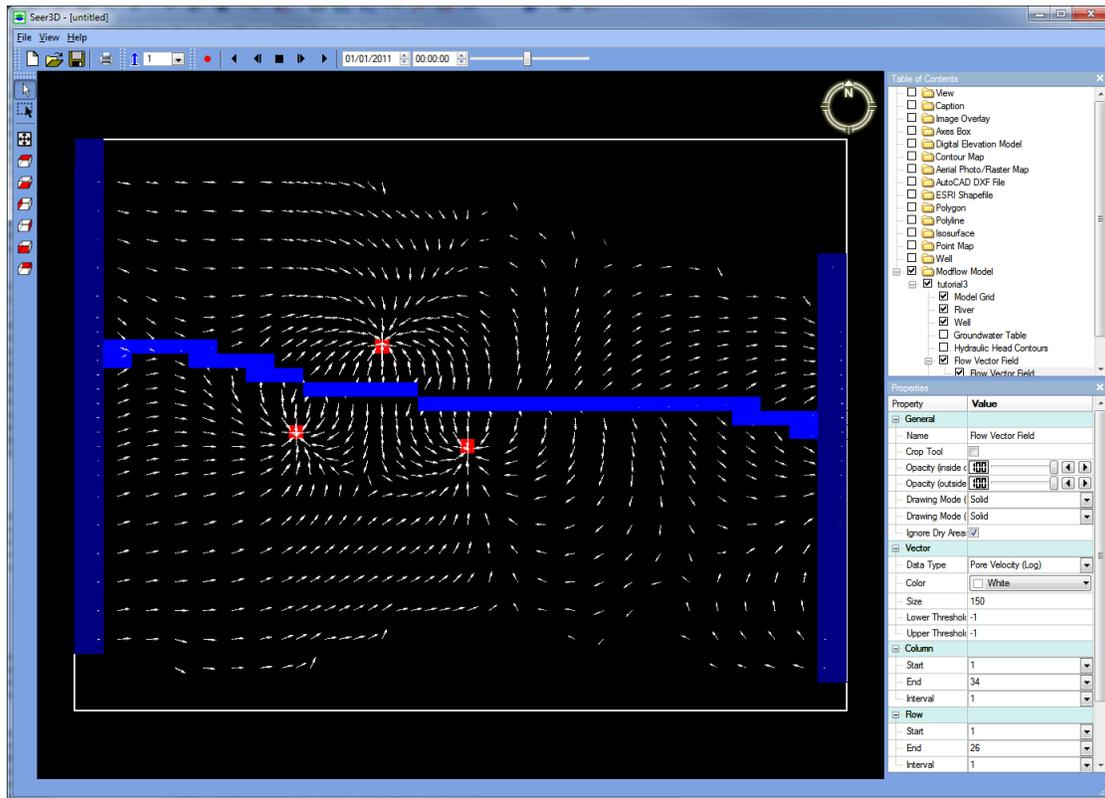
Figure 3.6. The flow field of model with flow vectors converge on three pumping wells represented by red rectangles.
