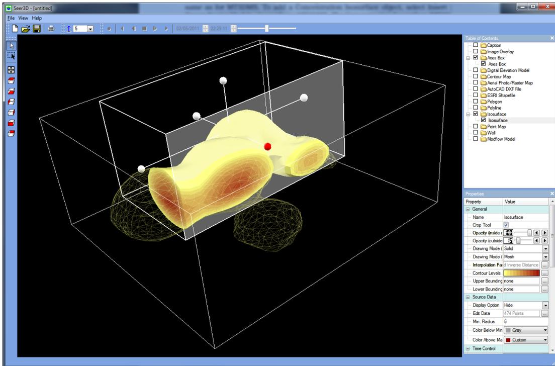
Figure 2.24. An isosurface with portions cropped away to reveal the concentration distribution
