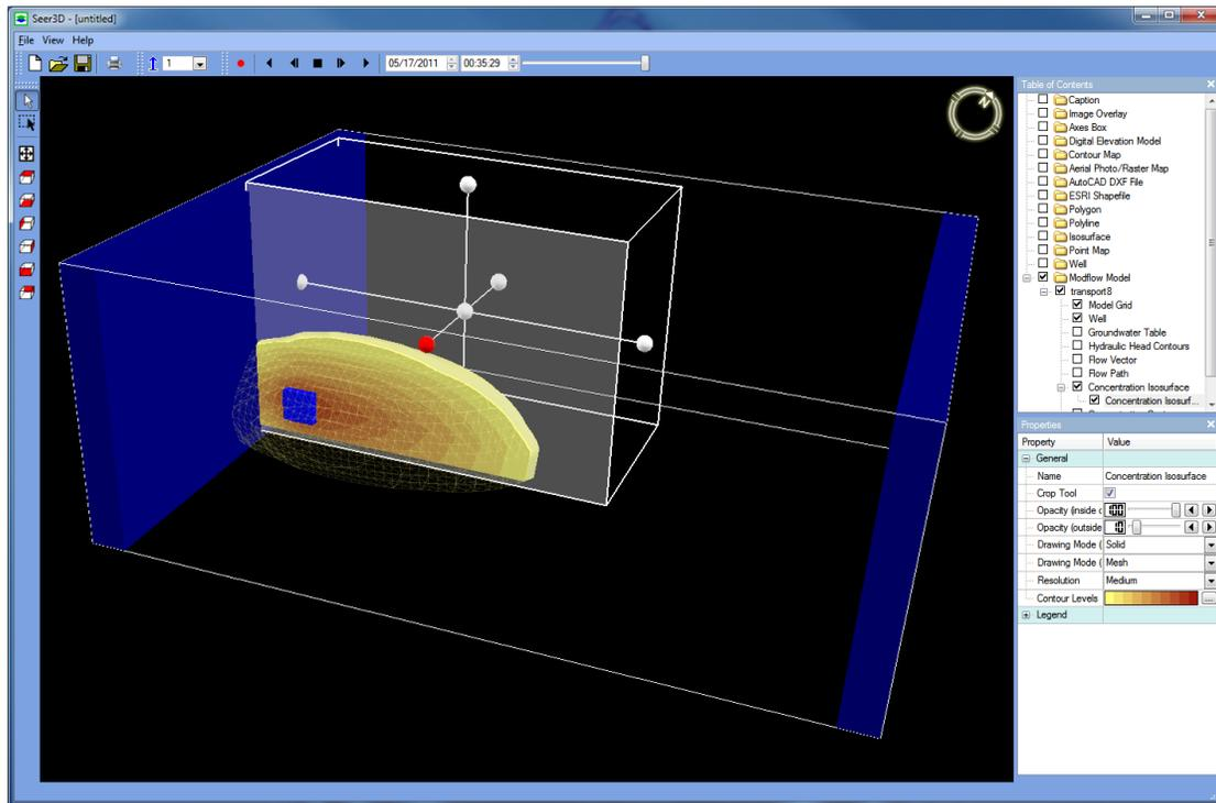
Figure 3.10. Concentration isosurface and contours based on the model results. The contours are automatically created on the face of the Crop Tool.
