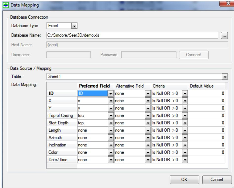
Figure 2.18. The Data Mapping dialog box for well data
