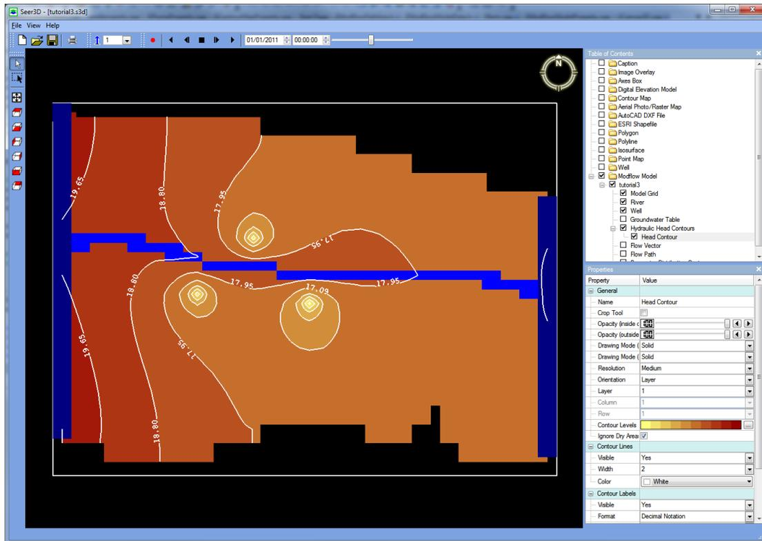
Figure 3.5. The Hydraulic Head Contours of a model
