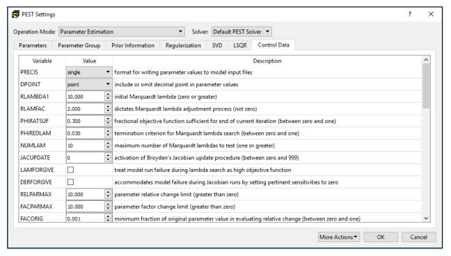
Figure 143. The Control Data tab of the PEST Settings dialog box
