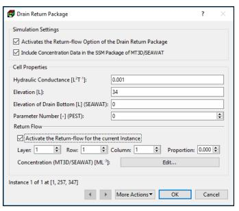
Figure 47. the Drain Return Package dialog box for specifying cell properties
