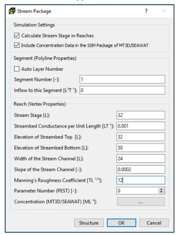
Figure 82. The Stream Package dialog box for specifying vertex properties
