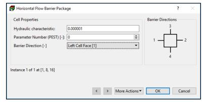
• Parameter Number is Figure 61. The Horizontal Flow Barrier Package dialog box used to group cells, where the hydraulic characteristic value is to be estimated by PEST. See *To define an*
