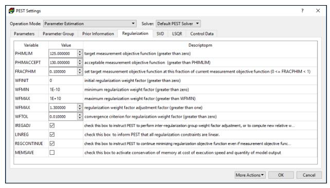
Figure 140. The Regularization tab of the PEST Settings dialog box
