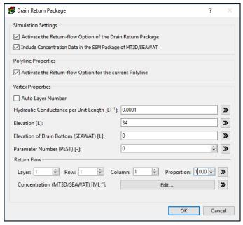
Figure 49. The Drain Return Package dialog box for specifying vertex/polyline properties
