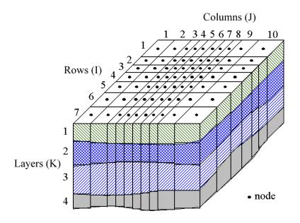
Figure 13. Spatial discretization of a Modflow Model
