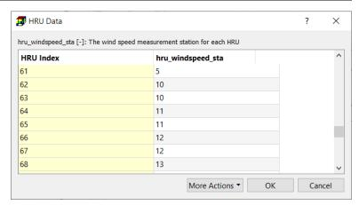
Figure 121. The HRU Data dialog box for wind speed stations
