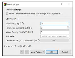
Figure 93. The Well Package dialog box for specifying cell properties
