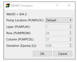
o Layer (PUMPLAY), Row (PUMPROW), Column (PUMPROL): These are the layer, row, and column numbers, respectively, of the cell (node) in this multi-node well where the pump intake (or outflow) is located. The location should correspond with one of the nodes specified in the MNW2 Nodes dialog box (Figure 70) for this multi-node well. These values are used only if PUMPLOC = By Layer.
