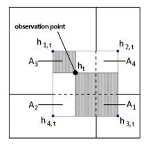
Figure 106. Interpolation of simulated head values to an observation point
