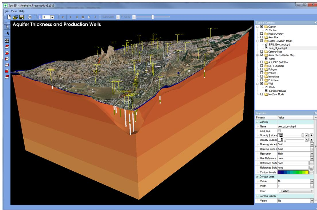
Figure 2.2. Digital elevation models used to depict aquifer thickness. Production wells and the well screens are displayed and an aerial photograph is draped on the ground surface to provide visual orientation
