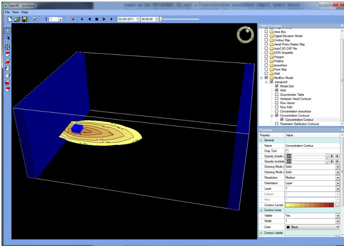
Figure 3.9. Concentration contours depicting results of a MT3DMS model
