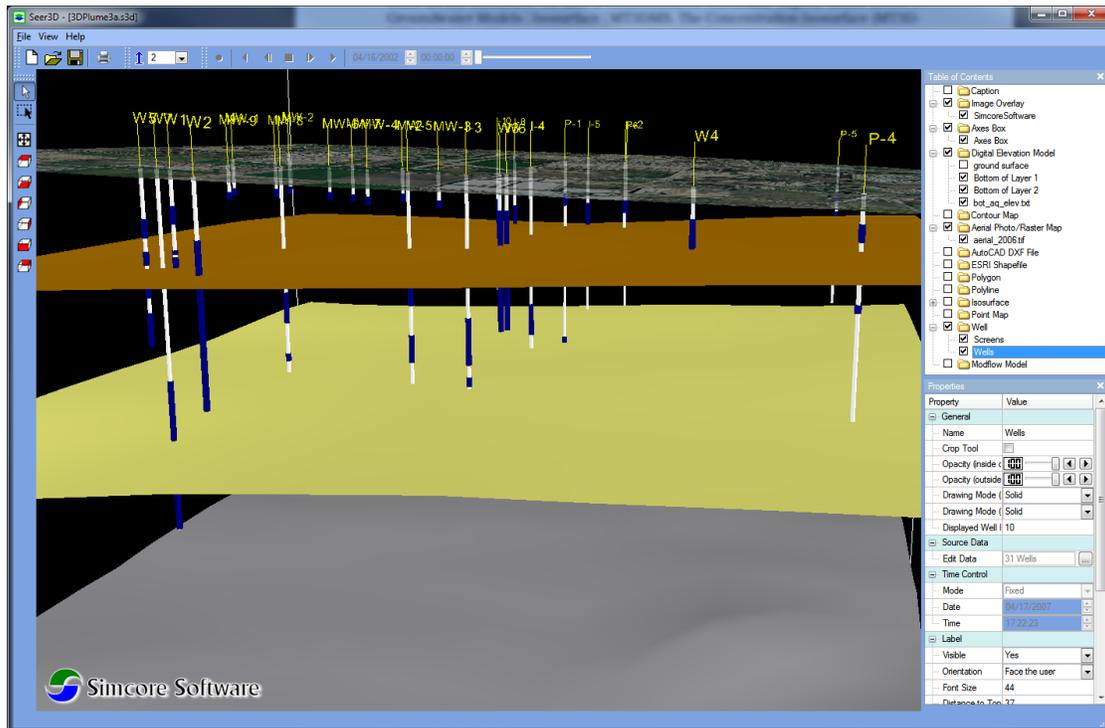
Figure 2.16. Wells penetrating several aquifer layers
